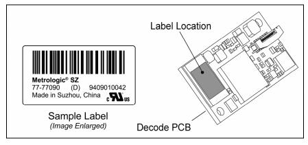
Figure 7. Decode Board (USB Version Shown) Serial Number Label Sample
